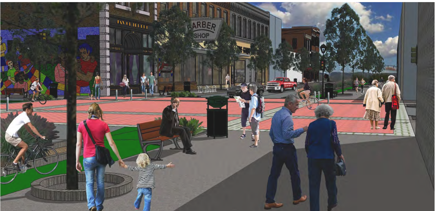
Figure 3.20: The Intersection of Tulare and L Street, looking towards Entertainment Plaza is the center of Downtown Dinuba. This design offers a pedestrian scramble, bollards, bulbouts and bioswale buffers between vehicular and bicycle traffic.
