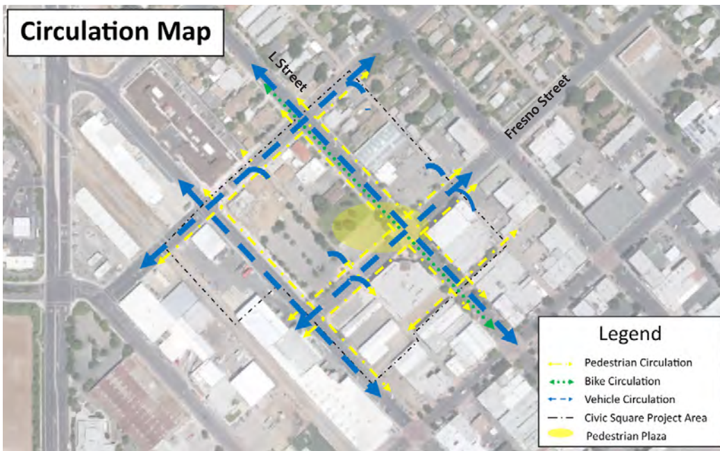
Figure 2.38: Circulation Map shows access to parking via alleys to reduce congestion along L Street
